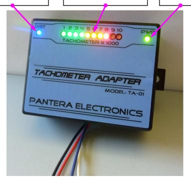
RED wire - connect to +12V when the ignition switch in the "RUN" position.
