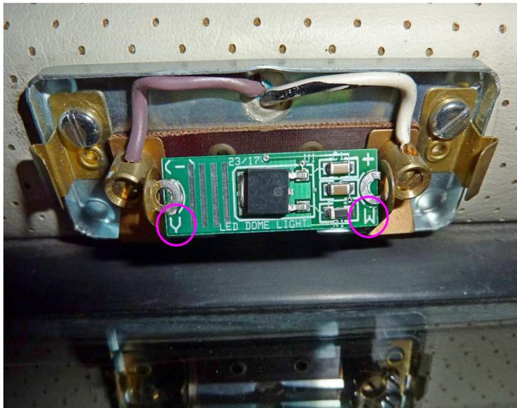
Rotate the LED Dome Lamp until the 2 LED's face outward.
