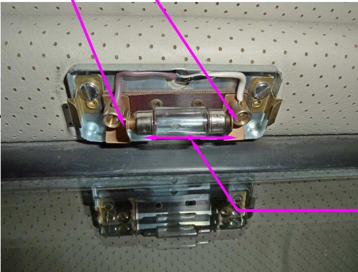
Remove the festoon bulb by gently push the bulb left or right.
