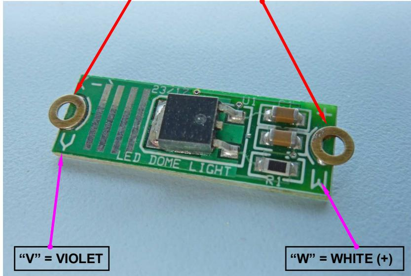
Insert one end of the LED Dome Lamp into one of the end springs and press it into the opposing spring. Your installation should look like the one below.
