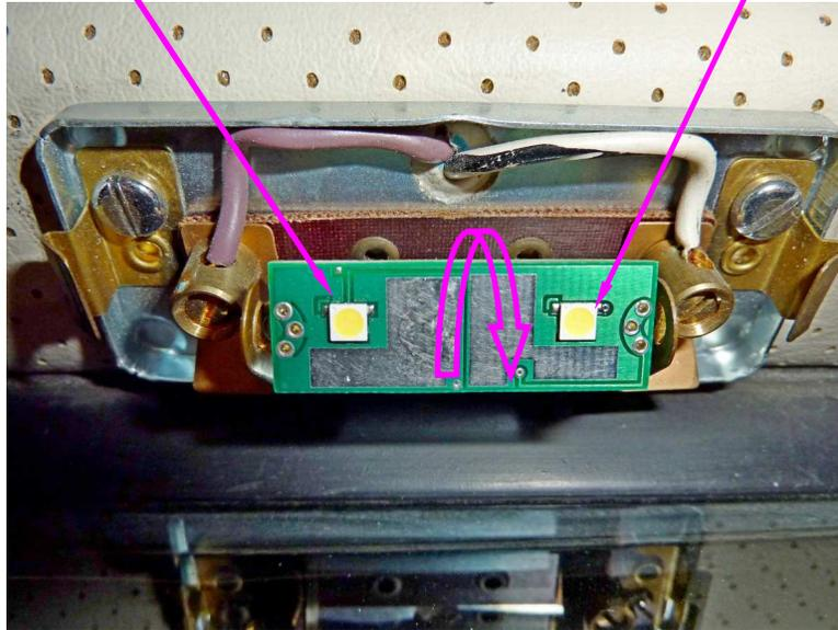
This is an installation in the console light used in 1973/74 Panteras. Note the "+" and "-" markings on the socket.
