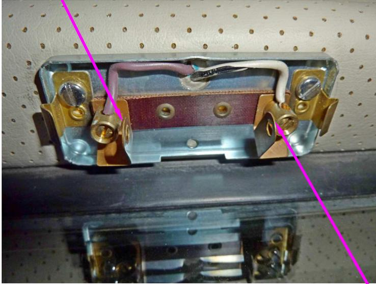
Install the LED Dome Lamp with the labeled end with a “+” and the letter “W”. This terminal is connected to the lamp socket with the WHITE wire.
