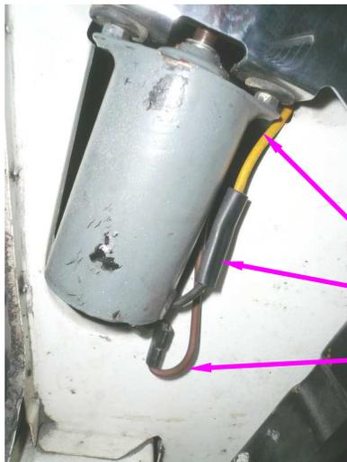
This is the correct factory wiring for the headlight lift motor. It must be wired in this configuration for the HMC to operate properly.
