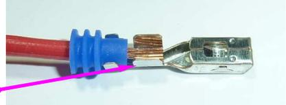
Assemble the terminal on the wire with seal.
