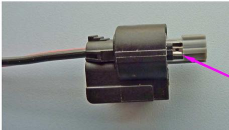
Push the terminal into the connector until it stops and the square hole in the terminal can be seen.
