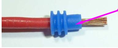
Slide the seal on the stripped section of the wire.
