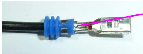
Crimp the assembly so that the seal and terminal look like in the picture.
