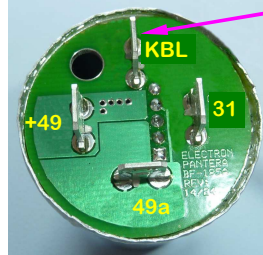
KBL terminal added to the original terminal layout.
