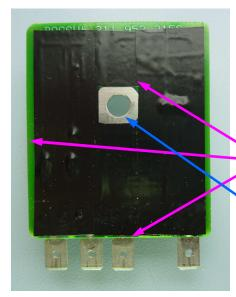
If the mounting surface is irregular or not flat it might be necessary to insulate the bottom of the replacement board.
