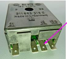
After pressing the board into the case the completed assembly should look like this with the terminals in this position.
