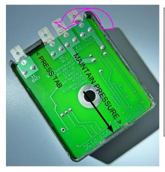
While maintaining pressure on the board to keep it in the slot press the board into the box.
