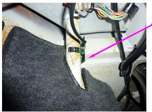
Mount the LED Footwell Lamp on the passenger side drain tube in the same manor.
