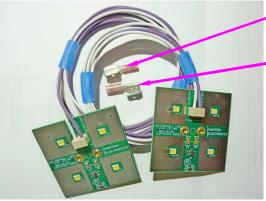
There are 2 piggy back terminals provided to connect the LED Footwell Lamps to the courtesy light switch and the fuse panel.
