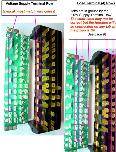
Terminal layout comparison of factory and ATO fuse panel, load terminal rows.
