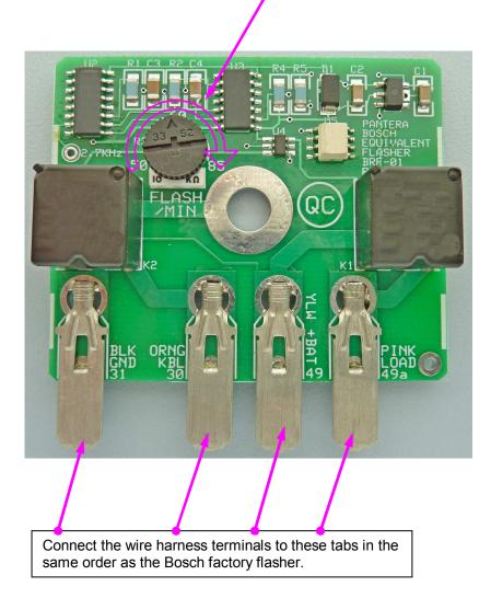
After adjusting the flash rate disconnect the wire harness connector and proceed with the board replacement.
