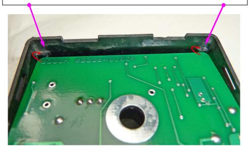
Lower the board while keeping the board sitting on the bosses and position the tabs in the slots. Make sure the board is flush with the edge of the case.
