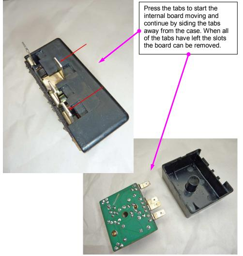
Place the replacement board into the case. Make sure the corners of the board sit on top of the bosses that are in the corners of the case.
