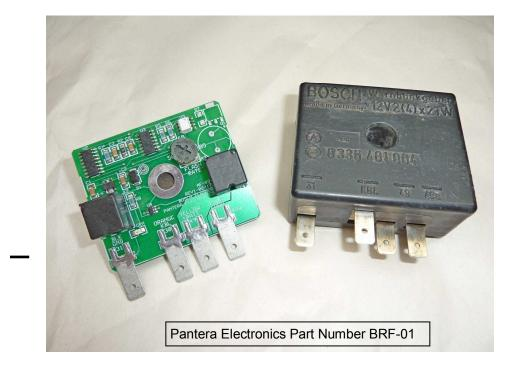
Before installing the replacement board the flash rate adjustment can be set by plugging in the harness and operation the flasher.
